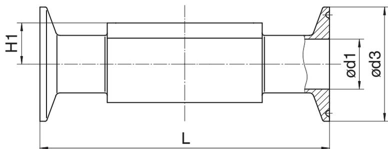
**Type de raccordement clamp DIN/ASME (code 80, 88, 8P, 8T)<sup>1)</sup>, inox forgé (code 40, 42, F4)<sup>2)</sup>**
