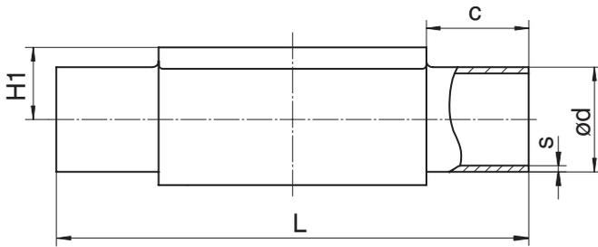
**Type de raccordement embout DIN/EN/ISO (code 0, 16, 17, 18, 60)<sup>1)</sup>, inox forgé (code 40, 42, F4)<sup>2)</sup>**
